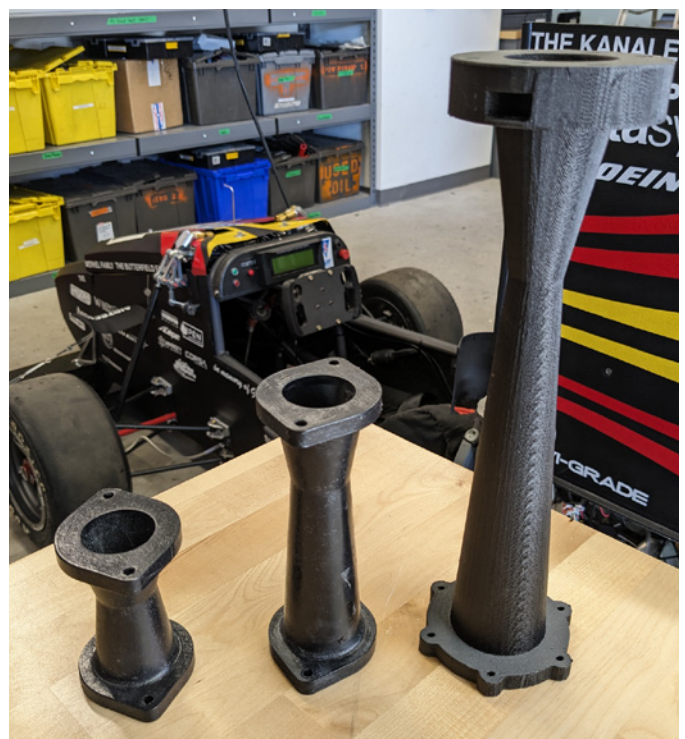
3D printed intake components.
